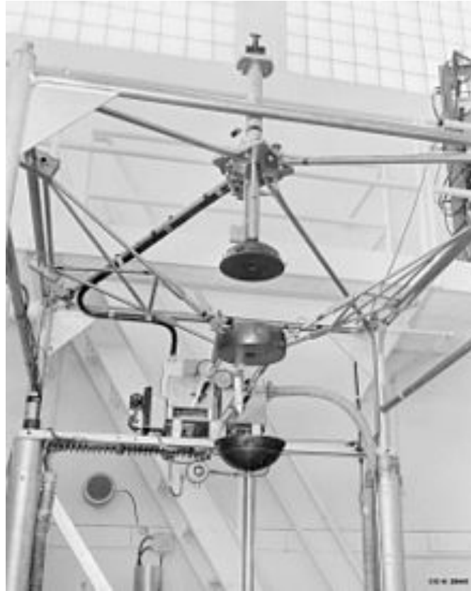
Figure 2.1: Lady Godiva Critical Assembly in a Scrammed Position.
